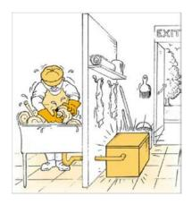
Grease traps: These are small devices connected directly to the outgoing drains of sinks inside the restaurant. Grease traps are designed to retain FOG usually from one fixture. Because they hold small quantities of captured FOG, such traps must be cleaned frequently.
