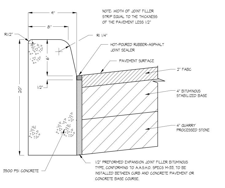
NOTE: TRANSVERSE JOINTS 1/2" WIDE SHALL BE INSTALLED 20'-0" APART AND SHALL BE FILLED WITH PREFORMED BITUMINOUS IMPREGNATED FIBER JOINT FILLER, COMPLYING WITH THE REQUIREMENTS OF A.A.S.H.O. SPEC. M-213, RECESSED 1/4" IN FROM FRONT FACE AND TOP OF CURB.
